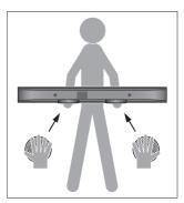
Handling the loudspeaker: In order not to dent or scratch the loudspeaker front grill, we recommend that you lift the loudspeaker by holding on to the two bass units on the bottom. Do not support the loudspeaker holding the loudspeaker front grill!
