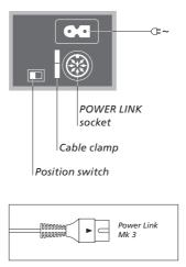
POWER LINK socket: Use this socket to connect the loudspeaker to one of the Power Link sockets on the Bang & Olufsen system.
