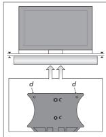
Adjustments: First, make sure that the television is adjusted to a level position on its stand! Then use the two screws (d) to adjust the loudspeaker so that it is parallel to the lower edge of the television. Align the loudspeaker front with the television and tighten the two screws (c).
